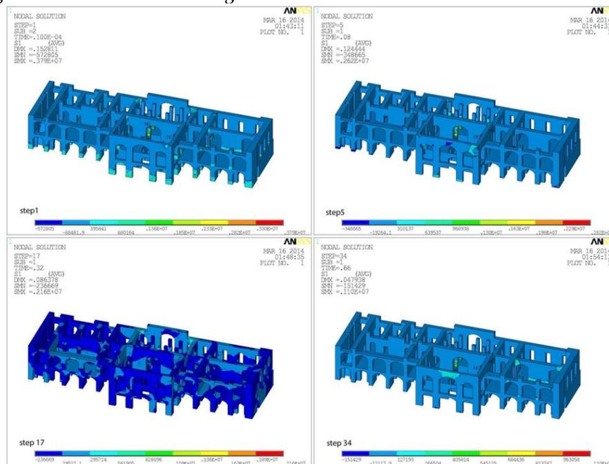
Fig. 3. The building under the effect of tensile stress in 1<sup>st</sup> analysis
