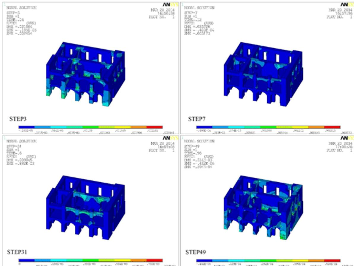
Fig. 6. One-third of the building after applying the separation distance under the tensile stress in the time-history analysis
