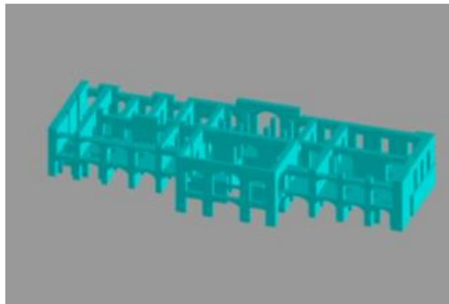
Fig. 1. Final volume of the courthouse building after modeling
